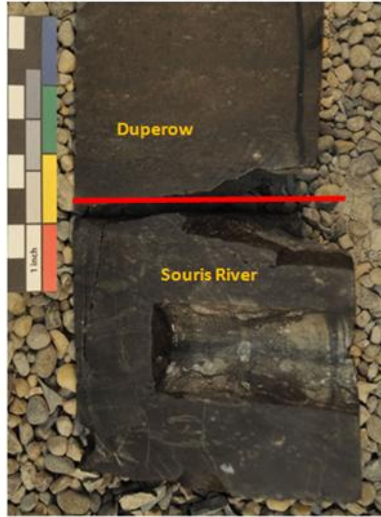
Figure 16. Contact of the Duperow and Souris River Formations, NDIC #9800, 10,955 ft.
