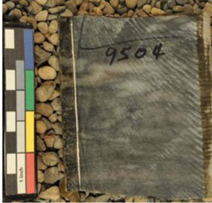
Figure 14. Anhydrite mottled with dolomite (LF7) core photograph. Gray to white crystalline anhydrite with variable amounts of dolomite, NDIC #2887,9,504ft.
