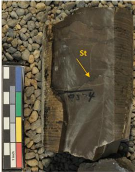
Figure 12. Dolomitic mudstone (LF5) core photograph. Dark brown to brown to stylolites (St), NDIC # 11005,9,374ft.
